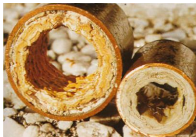
Limestone scaling of pipes
