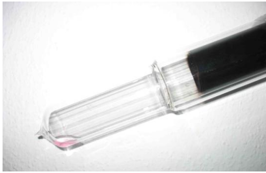
Condensation top of an all glass heat pipe (Here: for demonstration purposes in top-down position in order to show the heating liquid).
