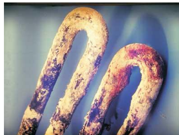
Scaling of electric rod.
